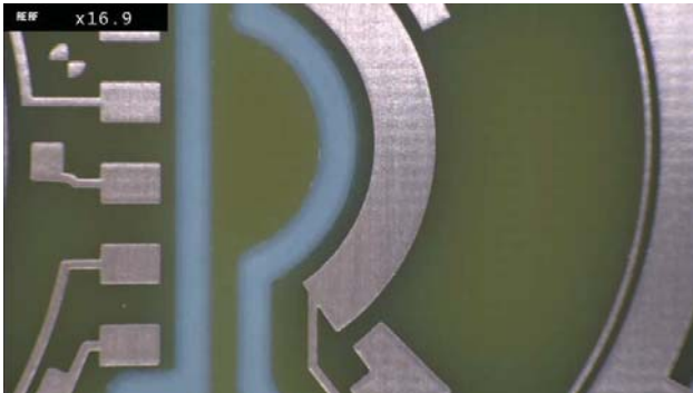
Process from PVI Nano Copper on FR4
